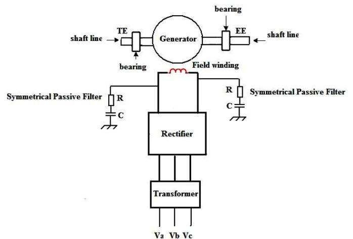
Fig. 3: Connection of the passive filter to the DC side of rectifier
