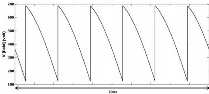
Fig .6: Field winding voltage in the case of applying the proposed passive filter
