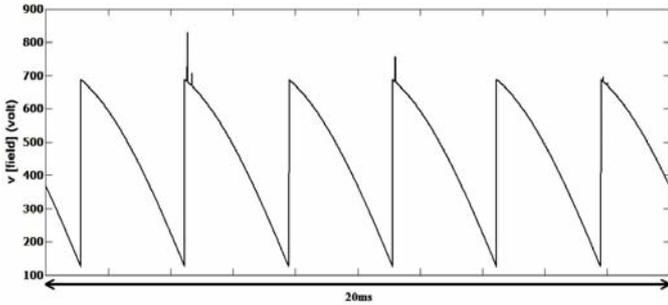
Fig .4: Voltage applied to the field winding of the proposed model
