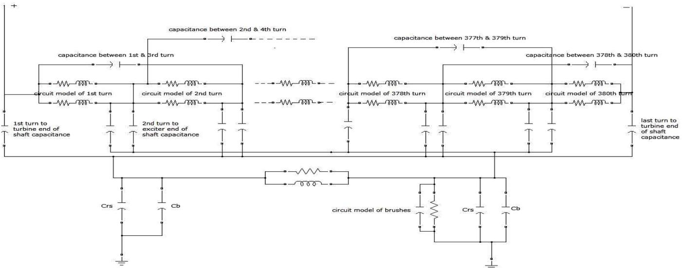
Fig. 2: Model of excitation winding and turbo shaft for ANSALDO 200MVA turbo generator
