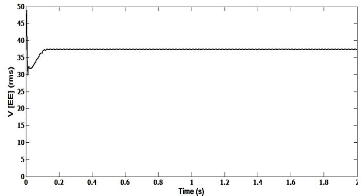
Fig .8: RMS value of shaft to ground voltage on the exciter end of generator
