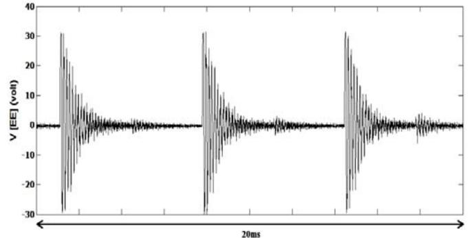
Fig .7: Shaft to ground voltage on (EE) in the case of applying the proposed passive filter
