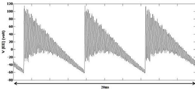
Fig .5: Shaft to ground voltage on (EE) without applying any solution
