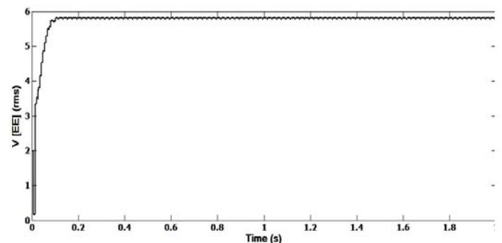
Fig .9: RMS value of shaft to ground voltage on the exciter end of generator in the case of applying passive filter
