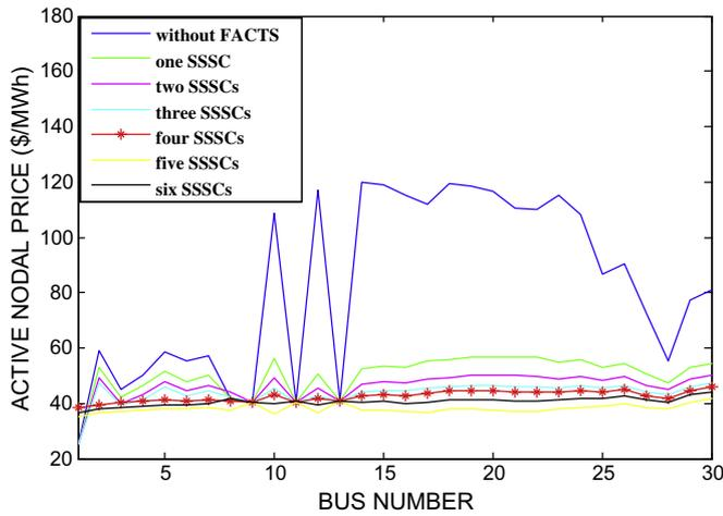
Fig. 5. Nodal prices of modified IEEE 30-bus test system with and without FACTS devices.
