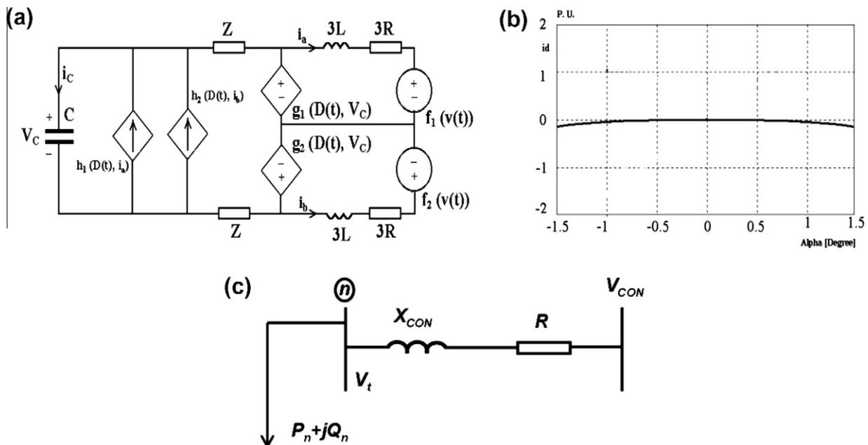
Fig. 1. (a) Average circuit model of STATCOM, (b) typical internal power losses of STATCOM obtained by the average model, (c) adaptation of the average model connected to the power system by adding a bus for STATCOM.
