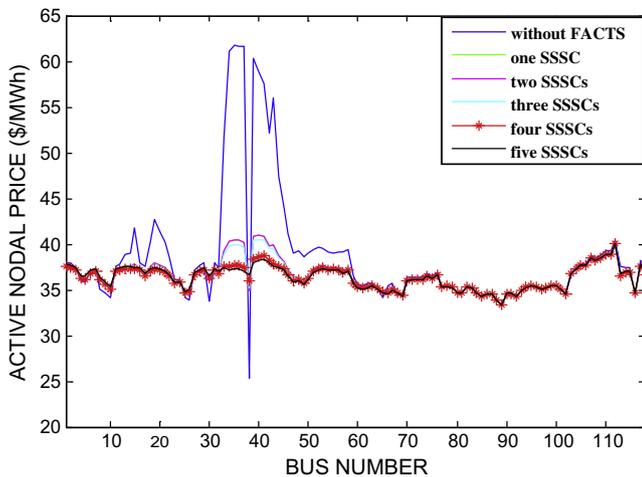
Fig. 6. Nodal prices of modified IEEE 118-bus test system with and without FACTS devices.
