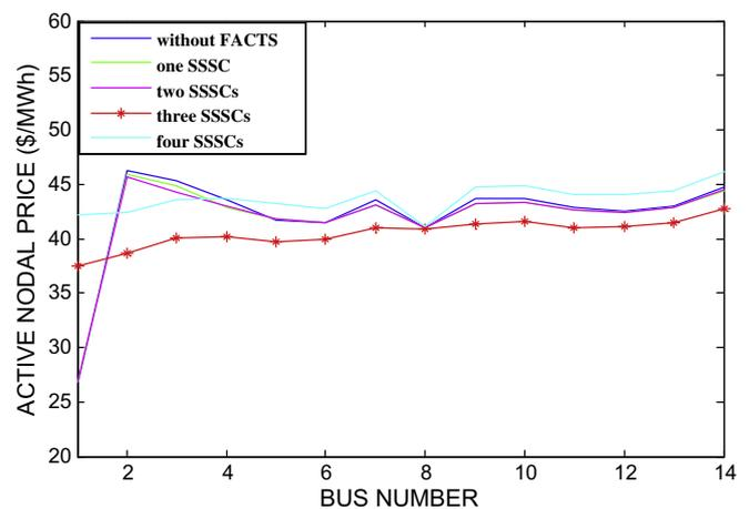
Fig. 4. Nodal prices of modified IEEE 14-bus test system with and without FACTS devices.
