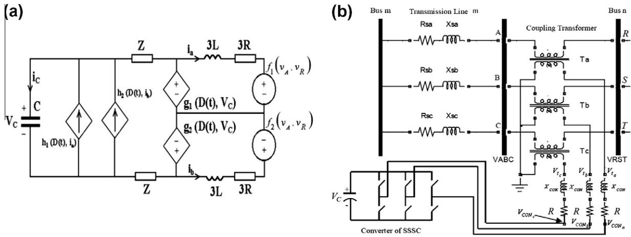
Fig. 2. (a) Average circuit model of SSSC and (b) three-phase circuit of SSSC.
